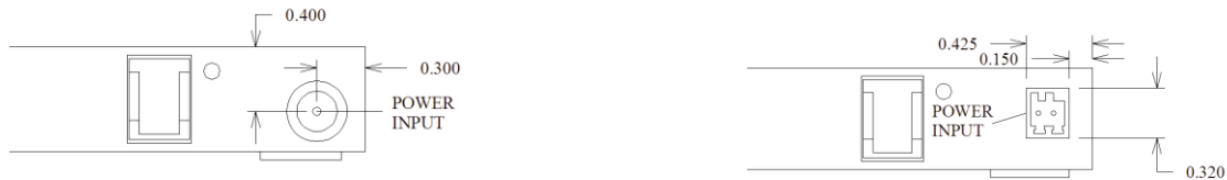
Figure 1: Power Configuration (12V AC 2.1mm P5 Connector on left, FlexPwr with Terminal Block Connector on right)
