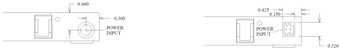
Figure 1: Power Configuration ( 12V AC with 2.1 mm P5 connector on left, FlexPwr with Terminal Block connector on right)
