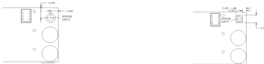
Figure 1: Power Configuration (12V AC 2.1mm P5 Connector on left, FlexPwr with Terminal Block Connector on right)
